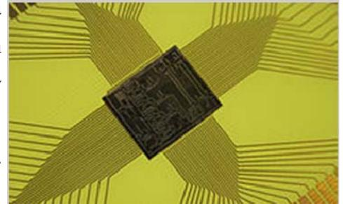
**Figure 1:** Microelectromechanical systems chip (lab on a chip).
